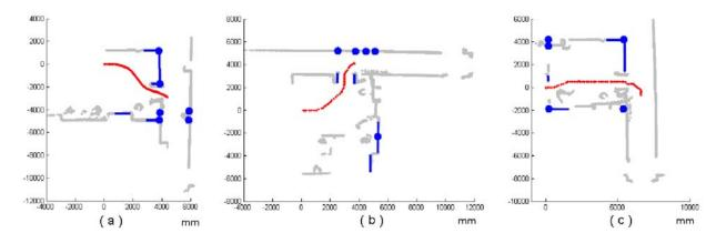
Fig. 5. Several tests in the same environment following different trajectories. The spectral clustering algorithm generates the same submaps in each experiment. When the robot leaves the room and enter in the corridor the thresholds values for *Ncut* and the second eigenvalue are satisfied.
