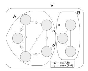
Fig. 3. This example illustrate two subsets  $A, B \subset V$  to show the concepts of *cut* and *assoc*. It can be noted how association involves not only the intergroup cohesion between A and B but the intragroup cohesion of the subset A (see text).
