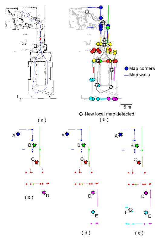
Fig. 6. Experiment in a real indoor environment with a laser range finder. a) Environment layout; b) detected submaps; c) submaps generated during the trajectory up to the third cut, d) and e) following partitions in the trajectory. Features have been obtained using a curvature-based laser scan data segmentation algorithm [17].
