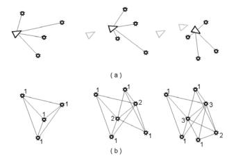
Fig. 1. Covisibility Graph building process. Each node is annotated with the number of observations of the corresponding feature. Edges represent locality of features and their values correspond to the times they have been observed simultaneously (these values have not been drawn).
