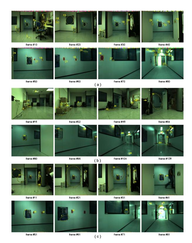
Fig. 7. Some experiments using vision. Three experiments in the same scenario in different viewing conditions. Visual landmarks detected are represented as ellipses, and the correspondence between landmarks in different frames with the corresponding index. A new area is detected at the same location as for the laser experiment. a) new area detected in frame #70, b) in frame #104 and c) in frame #71.
